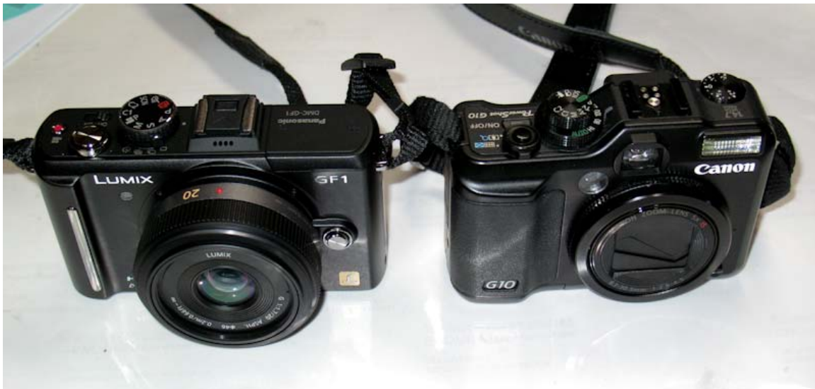
GF1 with 20mm (40mm equivalent) "pancake" lens and Canon G10 for size comparison.
